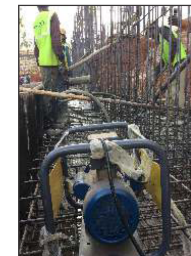
High Frequency Electric Vibrator 2800 rpm AME-2200M
